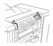
When removing the jammed media, be careful not to touch the transfer belt. Touching the transfer belt may result in decreased print quality.
