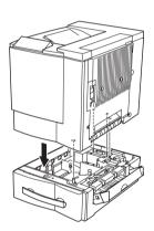
11 Install the brackets (two at the front and one at the back), and then close the right door.
