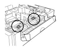
9 Wipe the paper feed rollers inside the right door with a soft, damp cloth.
