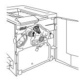
2 Grasp the release lever for the OPC drum cartridge, and then pull the cartridge straight out about 6 inches (152 mm).
