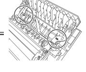
**d** Open the duplex option's cover and tighten the two thumbscrews on the duplex option to secure the unit to the printer.
