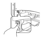
2 Remove the cover from the right side of the printer. Use a Phillips screwdriver to remove the two screws securing the right cover.
