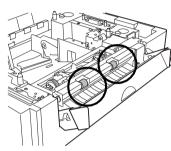
10 With the right door still open, place the printer on the lower feeder unit.
