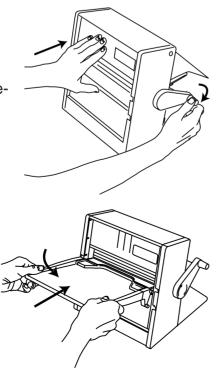
Install feed tray and trim off excess film using cut blade.
