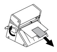
Install feed tray and trim off excess film using cut blade.
