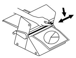
Step 3 - Trim to desired length using the cut blade at the roller exit. Apply pressure down on the orange blade holder and slide to the left or right.
