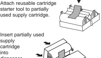
cartridge into dispenser. Note: tool should be positioned between rubber rollers in dispenser.
